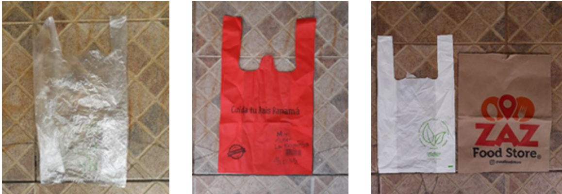
Figure 7: Example of traditional PE (left) and PP (middle) grocery bags and compostable PLA and paper alternatives (right) offered at grocery stores in Panama City
